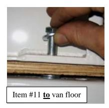
On 3<sup>rd</sup> Compartment Doorframe repeat the same steps done on Rear Doorframe. Only one bolt is used and must be located just to the left of the doors hinge as shown above.
